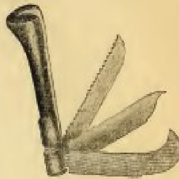
Larger Knife, without spring, kept open or shut, by turning a ferrule.
